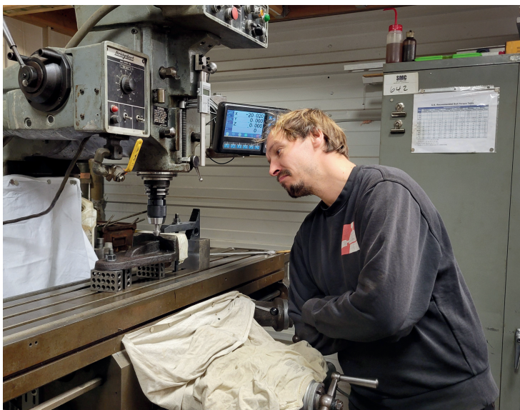
Erik using Colton Juelsgaard's machine to drill new holes in the cast iron sliders
