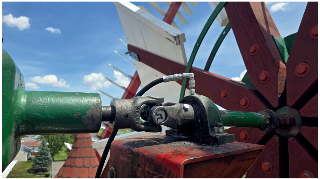
The repair Mike Mortensen made to the fantail axle
